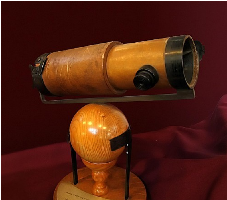
This is a replica of Newton's reflecting telescope. Newton's redesign of the telescope became the basis for the space-based Hubble telescope and most other large modern telescopes both on the ground and in space. (commons.wikimedia.org)
