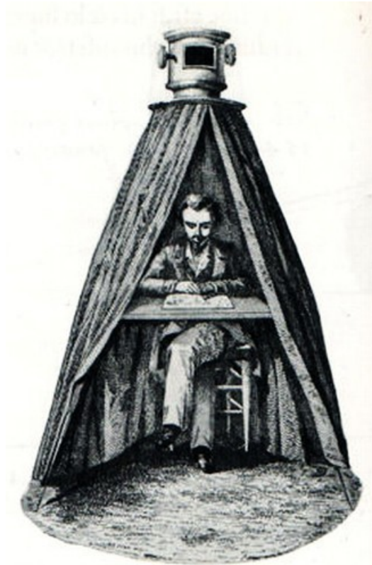
A drawing of a Kepler movable tent-type camera obscura -- the type designed by Kepler in 1620. (commons.wikimedia.org)
