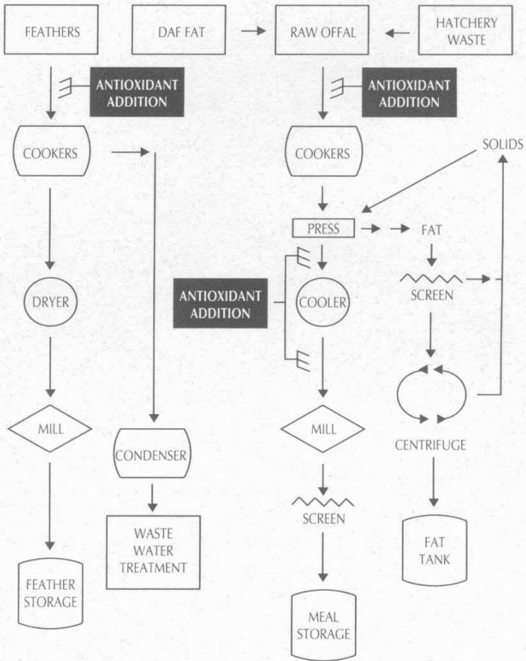
**Figure 1. Flow chart of a rendering plant and proposed sites for the addition of antioxidants**
