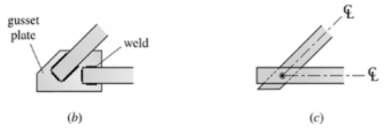
Truss Definitions and Details
