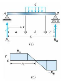
for a < x < a + b  $V = R_A - q(x - a)$   $M = R_A x - q(x - a)^2 / 2$   $M_{\text{max}}$
