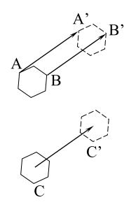
Sliding vector A vector whose *line of action* must be specified in addition to its *magnitude* and *direction*. For example, external force/moment acting on the rigid body.
