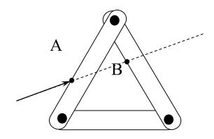
Fixed vector A vector whose *magnitude*, *direction*, *line of action*, and *point of application* are all important. For example, external force/moment applied onto the nonrigid body. Deformable effect of the object is important.
