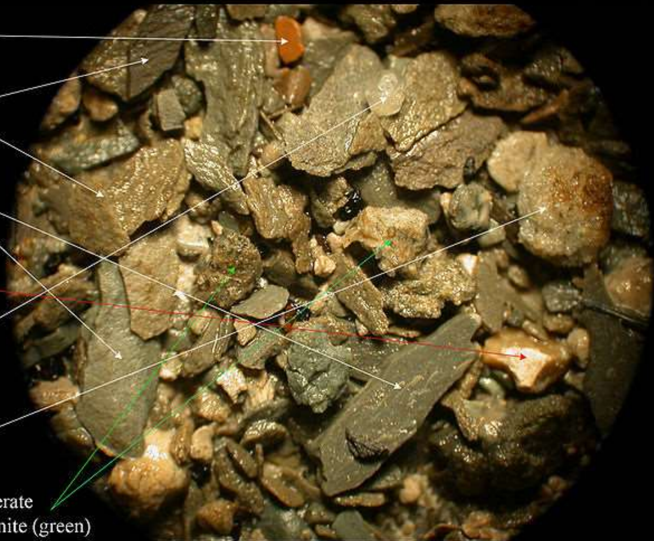
Sample of drill cuttings under a 10x microscope
