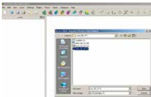
Figure 23: Adding the Digital Elevation Model data as raster layer in QGIS
