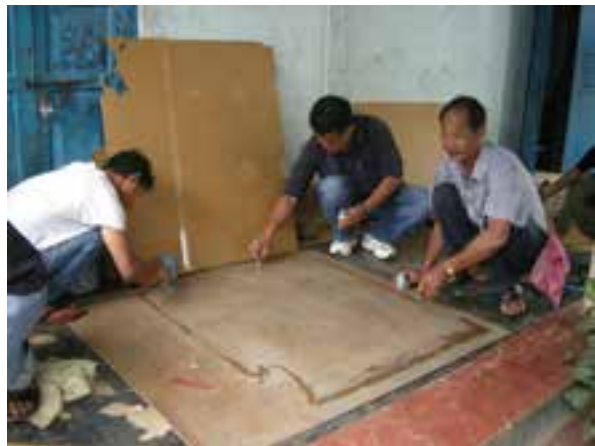
Figure 42: Gluing of plywood model base
