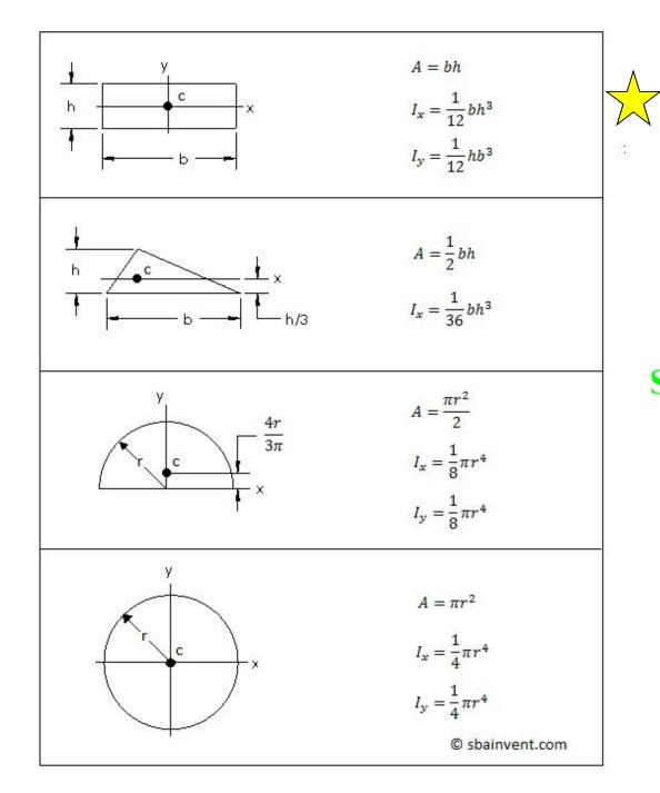
Moment of Inertia of Some Basic Geometric Shapes
