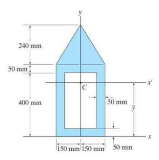
A composite area is made by adding or subtracting a series of "simple" shaped areas like rectangles, triangles, and circles.
