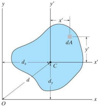
This theorem relates the moment of inertia (MoI) of an area <u>about an axis</u> <u>passing through the area's centroid</u> to the MoI of the area about a <u>corresponding parallel axis.</u> This theorem has many practical applications, <u>especially when working</u> <u>with composite areas</u>.
