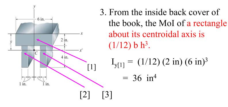
Using the parallel-axis theorem,
