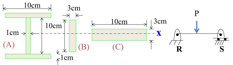
Consider three different possible cross sectional shapes and areas for the beam RS. All have the same total area and, assuming they are made of same material, they will have the same mass per unit length.
