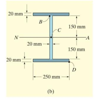
Find the moment of inertia of the section shown with respect to the neutral axis (NA).
