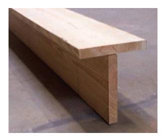
Cross-sectional areas of structural members are usually made of simple shapes or combination of simple shapes. To design these types of members, we need to find the moment of inertia (MoI).
