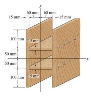
This is another example of a structural member with a composite cross-area. Such assemblies are often referred to as a "builtup" beam or member.
