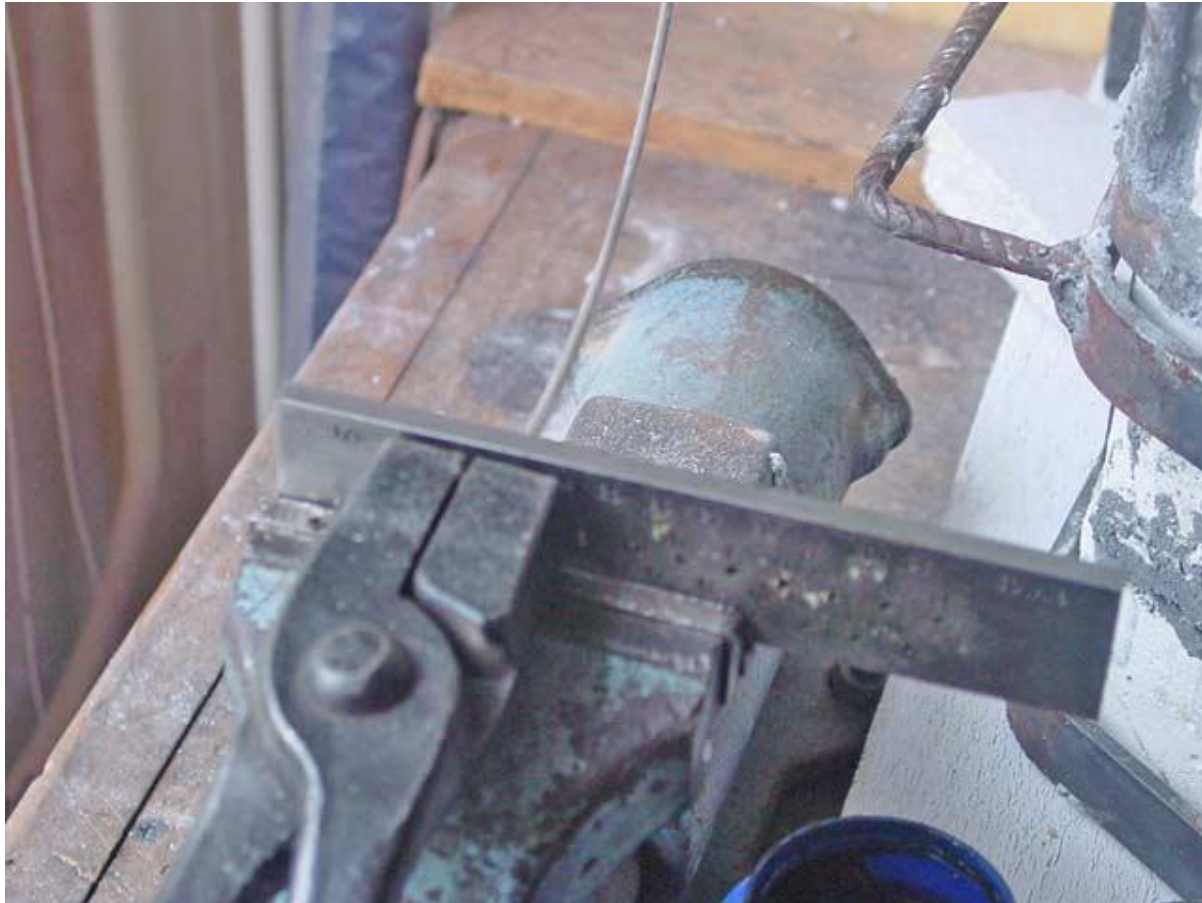
Fig: 3.7 Drawing silver wire by hand pulling
