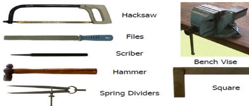
Fig 4.9 Marking and measuring tools
