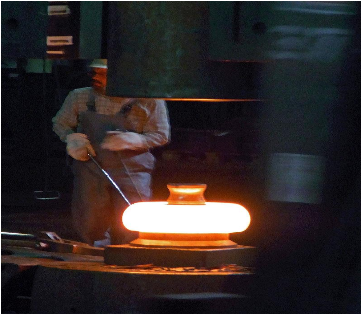
FIG: 2.16 OPEN-DIE DROP FORGING (WITH TWO DIES) OF AN INGOT TO BE FURTHER PROCESSED INTO A WHEEL
