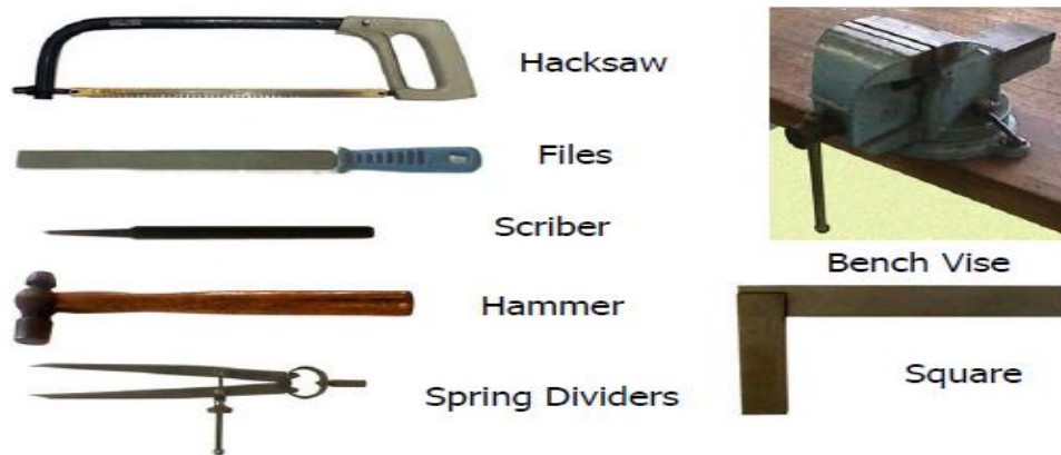
Fig 4.15 Marking and measuring tools
