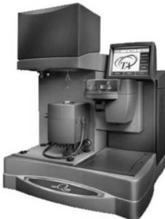
Fig.9. A TGA Instrument
