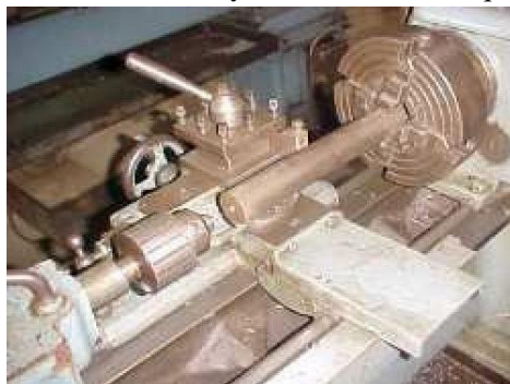
Fig. 2.24 Holding drill chuck and drill in tailstock
