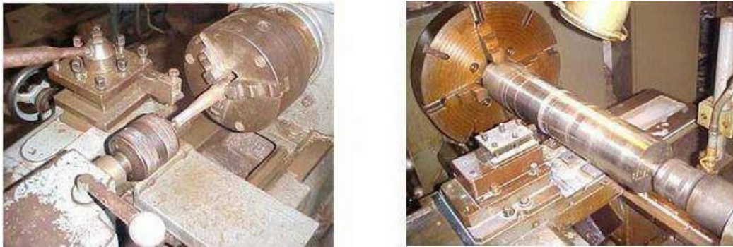
Fig. 2.19 Work held between chuck and revolving centre
