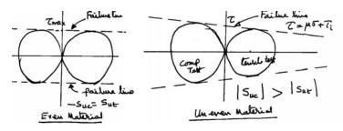
The lines tangent to these circles constitute failure lines for all combinations of applied stress between the two circles. The area enclosed by the circles and the failure lines represent a safe zone.
