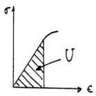
Let  $U_h$  be energy due to volume change and  $U_d$  be energy due to distortion. Then we can express each of the principal stresses in terms of hydrostatic component ( $\sigma_h$ ), common to all the faces of volume element and distortion component ( $\sigma_{id}$ ) that is unique to each face.
