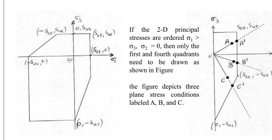
Point A represents any stress state in which the two non zero principal stresses  $\sigma_1$ ,  $\sigma_3$  are positive. Failure will occur when the load line OA crosses the failure envelop at A'The safety factor for this situation can be expressed as
