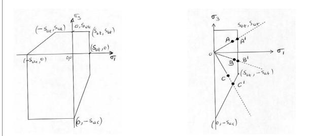
If the two nonzero principal stresses have opposite sign, then two possibilities exist for failure, as depicted by points B and C. The only difference between these two points is the relative values of their two stress components  $\sigma_{1,}$  and  $\sigma_{3}$ . The load line OB exits the failure envelop at B' above the point( $S_{ut}$ ,- $S_{ut}$ ) and the safety factor for this case is the same as the previous equation.
