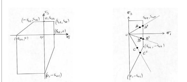
If the stress state is as depicted by point C, then the intersection of the load line OC and the failure envelop occurs at C' below the point  $(S_{ut}, -S_{ut})$ . The safety factor can be found by solving for the intersection between the load line OC and the failure line and is given by
