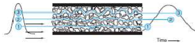
FIGURE 22-20 Band spreading from multiple flow paths. The smaller the stationary phase particles, the less serious this problem is. This process is absent in an open tubular column. (Adapted from H. M. McNair and E. J. Bonell, Basic Gas Chromatography (Palo Alto, CA: Varian Instrument Division, 1969).)
