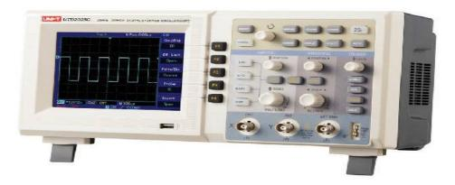
Its screen has two dimensional graph plotting ability. Vertical is for Voltage, and Horizontal is for Time.
