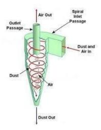
The denser dust particles in the rotating air stream will have more inertia than the air molecules. So dust particles will not able to follow the spiral curve of the air flow. Instead they will strike with the wall and will fall down in the bottom of the conical shape container. In a conical system, as the rotating flow moves towards the narrow end of the cyclone the rotational radius of the stream is reduced which helps in separating smaller and smaller particles.
