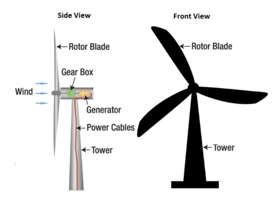
Two or three-blade wind turbines are now used almost exclusively for the production of electric power. The main parts of the systems that comprise these wind turbines are
