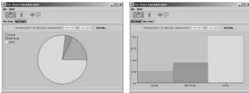
Figure 3.3 Java Pet Store Sample Application Administrator Client Displaying Order Data in Pie and Bar Charts Using the JFC/Swing API
