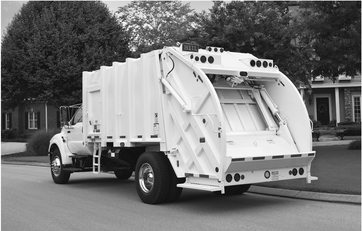
FIGURE 11-5 Typical rear-loading refuse collection vehicle. (Source: Heil Environmental, 2006.)
