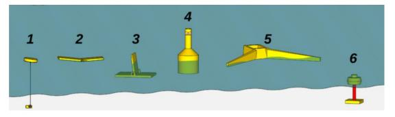
An example of a surface attenuator is the *Pelamis Wave Energy Converter*. By floating on the waves, this machine converts *the energy in the wave into mechanical energy*, and subsequently into electrical energy.
