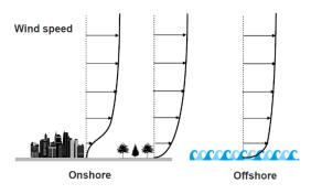
slowed down by the presence of buildings, trees, etc. This means that the *wind* speed will reach a fairly *constant* value at a much higher altitude than offshore. In short, *offshore* wind turbines generally benefit from much stronger and *uniform* winds.
