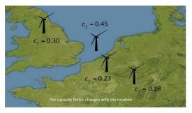
It should be kept in mind that a very *large capacity factor* is not necessarily the *economic optimum*. For example, in a given wind, a *smaller wind turbine* might have a larger capacity factor than a *large wind turbine* but eventually produce less power. Imagine that the wind speed varies between 10 m/s and 20m/s at a given location. Placing let's say a *IMW* turbine at this location
