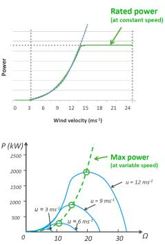
generator torque, and is therefore called *torque control*. Eventually, when *rated power* is *attained*, the *power* is *kept constant* by turning the blades along their axis, that is by *pitching* them.
