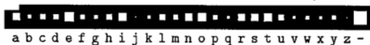
Figure 1.16. Probability distribution over the 27 outcomes for a randomly selected letter in an English language document (estimated from The frequently asked questions manual for Linux ). The picture shows the probabilities by the sizes of white squares.
