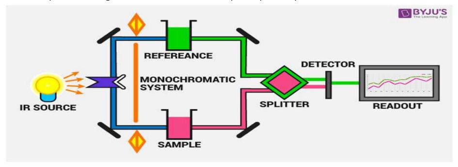
Now, both of these beams are reflected to pass through a splitter and then through a detector. Finally, the required reading is printed out after the processor deciphers the data passed through the detector.
