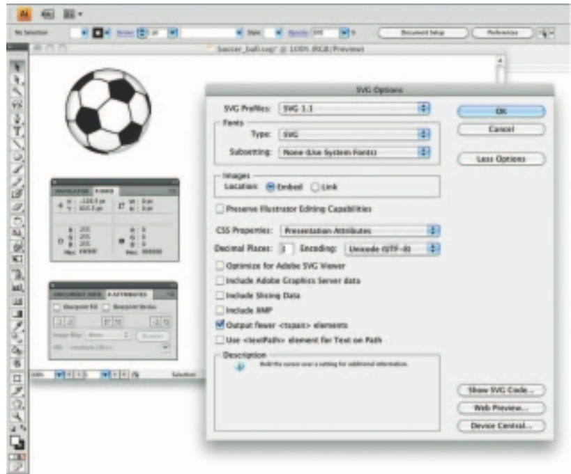
Figure 3-8 Drawing software such as Adobe Illustrator can save vector graphics in SVG format.
