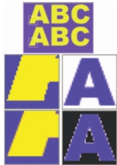
Figure 2-9 Anti-aliasing text and graphics creates “smooth” boundaries between colors. The top row of letters is not anti-aliased; the bottom row is.
