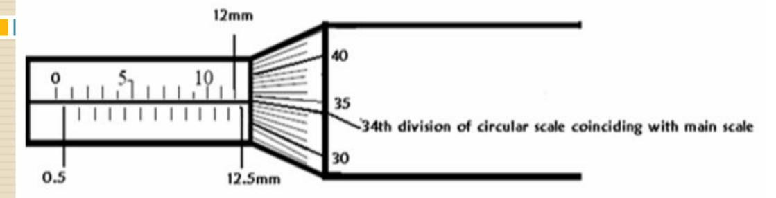
Formulae of calculating total reading with the help of outside micrometer is
