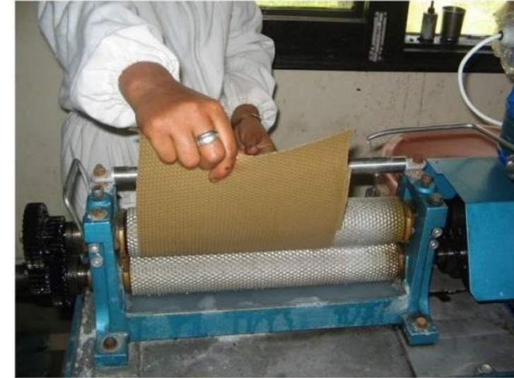
Comb Foundation Mill
