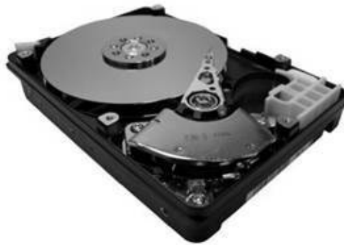
Picture 21: Hard disk internal mechanical construction
