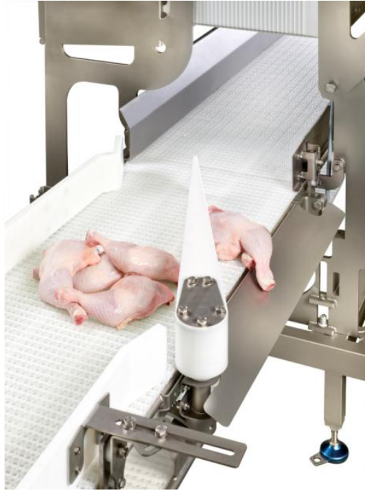
Figure 5.17.1 An example of an automated sorting station. This is done after weighing each piece on another short segment of the belt (i.e., a standalone segment equipped with a fast weighing system). The weighing station is located about 5-10 meters in front of the sorting station, so there is enough time for data processing and execution. Courtesy of Marel.
