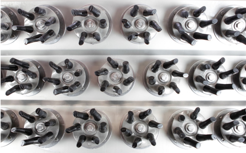
Figure 5.7.1 De-feathering disks mounted on a vertical surface. The birds are moved in between disks mounted on both sides; distance can be adjusted to accommodate different size of birds. Courtesy of Stork.
