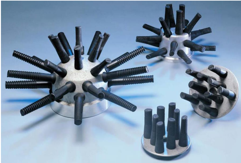
Figure 5.7.2 Examples of different fingers and disk mounting for de-feathering equipment.
