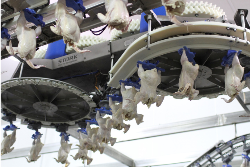
Figure 5.10.1 An example of an automatic bird weighing system which also includes a temporary transfer system. Courtesy of Stork.
