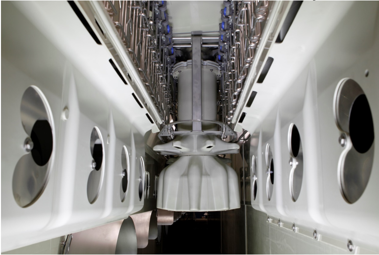
Figure 5.6.2 A new steam scalding system showing the shackle line (top) and the strategic location of the vents for the steam discharge (sides). Courtesy of Marel.
