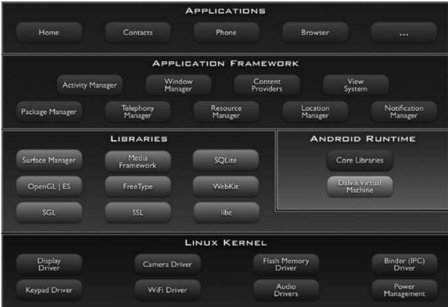
Figure 9.4 Major components of the Android operating system. (Source: http://d.android.com/guide/basics/what-is-android.html .)
