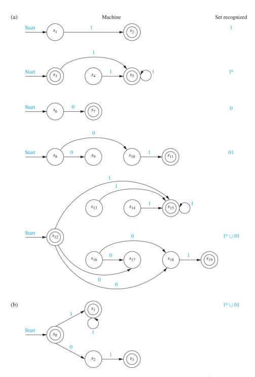
**FIGURE 3** Nondeterministic finite-state automata recognizing  $1^* \cup 01$ .
