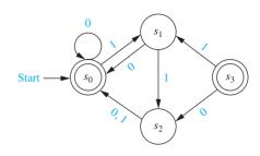
FIGURE 1 The state diagram for a finite-state automaton.
