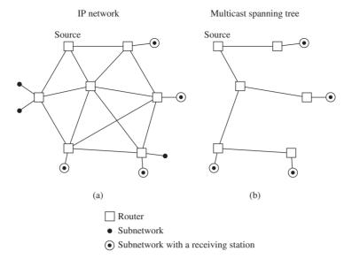
FIGURE 5 A multicast spanning tree.
