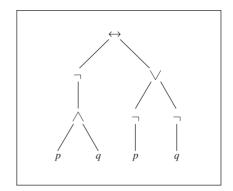
FIGURE 14 Constructing the rooted tree for a compound proposition.
