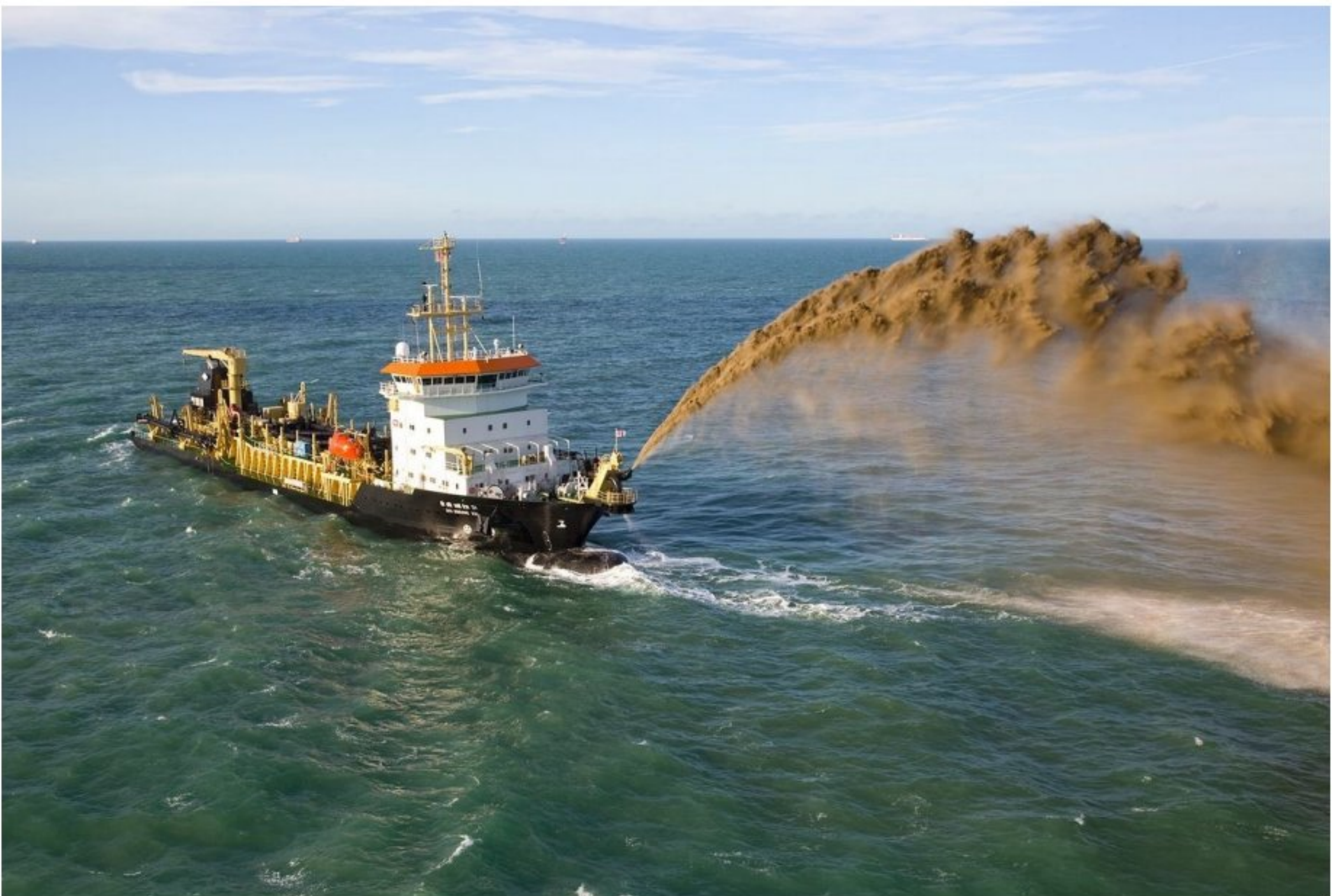
Fig. 12. Unloading of sample material during dredging process.
