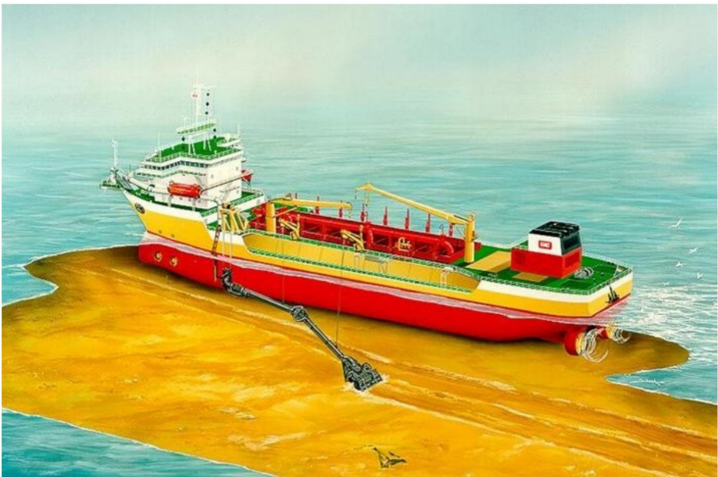
Fig.10. Ocean floor dredging using one pipe. Image source:
