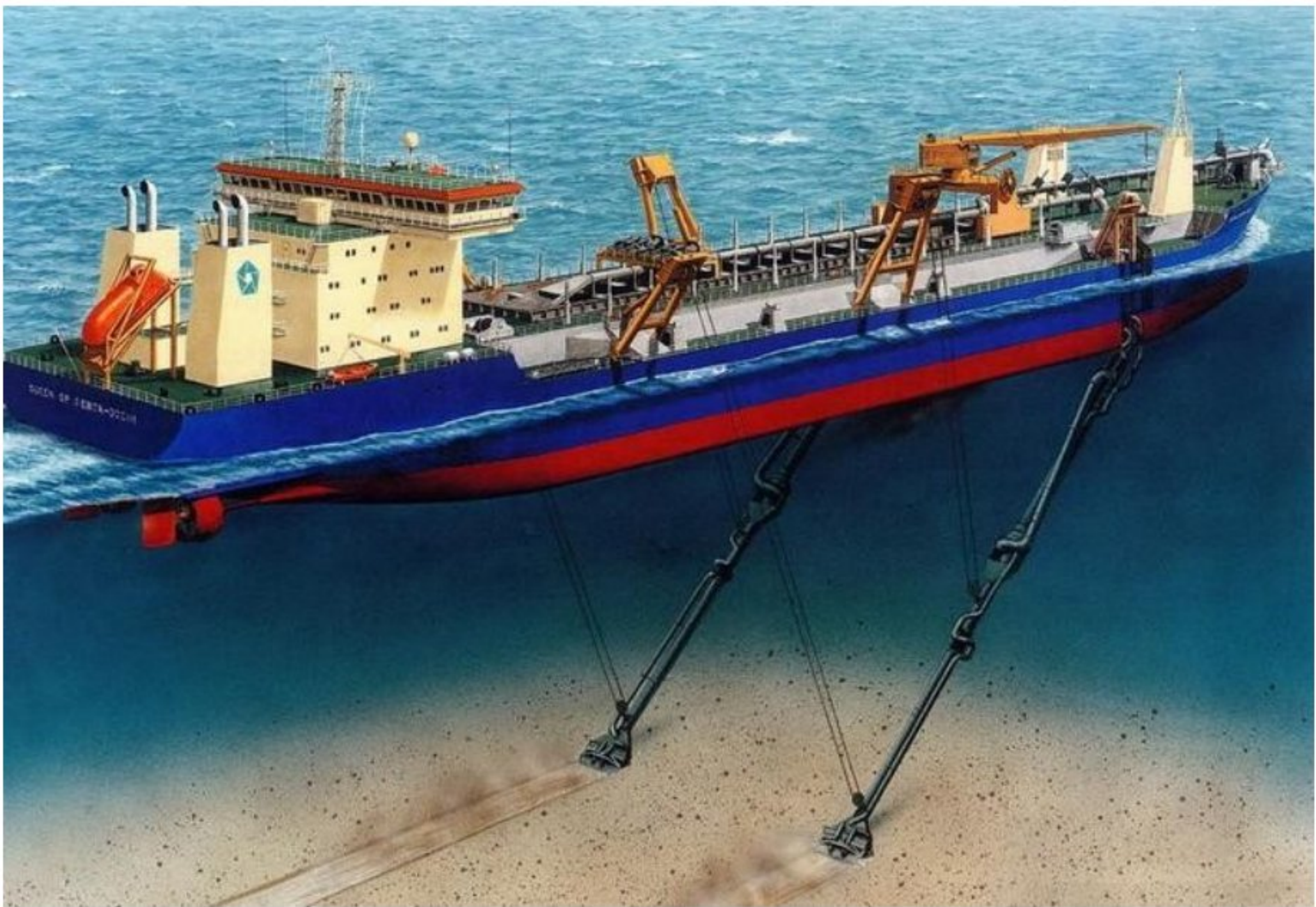
Fig.11. Ocean floor dredging using two pipes. Image source:
