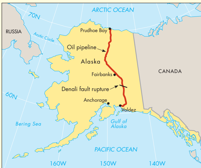
Figure 6.E A Trans-Alaska oil pipeline survives (M 7.9) earthquake The Alaskan pipeline was designed to withstand several meters of horizontal displacement on the Denali fault. The 2002 earthquake caused a rupture of 4.3 m (14 ft) beneath the pipeline. The built-in bends on slider beams with teflon shoes accommodated the rupture as designed. This was strong confirmation of the value of estimating potential ground rupture and taking action to remove the potential threat and damage. [Alyeska Pipeline Service Company (ASPC)]
