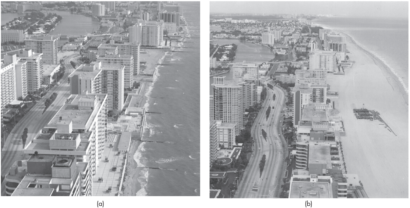
Figure 10.13 Beach nourishment Miami Beach (a) before and (b) after beach nourishment. (Courtesy of U.S. Army Corps of Engineers)
