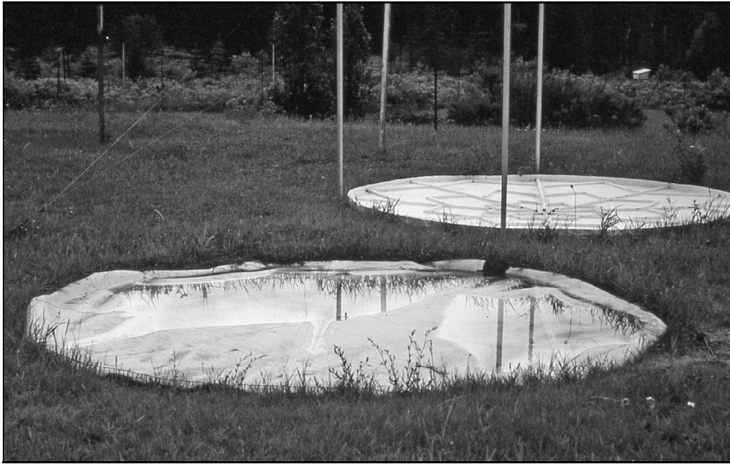
Figure 5.10 A snow pillow (foreground) and a water-output lysimeter (background) installed at the US National Weather Service snow-research site at Danville, Vermont. Buried lines transmit the fluid pressure from the pillow to a sensor, and the water released by the snowpack to a measuring device, both of which are in an instrument shelter. The metal ring is electrically heated, and is melted down through the snowpack to isolate the cylinder of snow above the lysimeter (photo by author).
