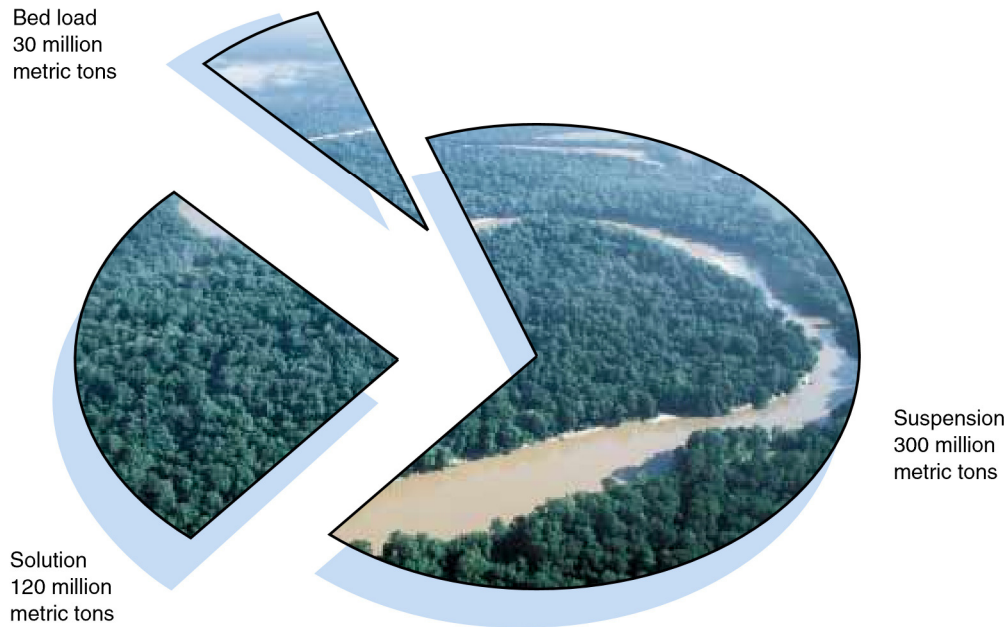
Figure 14-8 The Mississippi River carries the greatest proportion of its sediment as suspended load. Numbers indicate sediment load per year.
