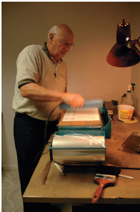
Document examiner using Electrostatic Detection Apparatus to develop written impressions
