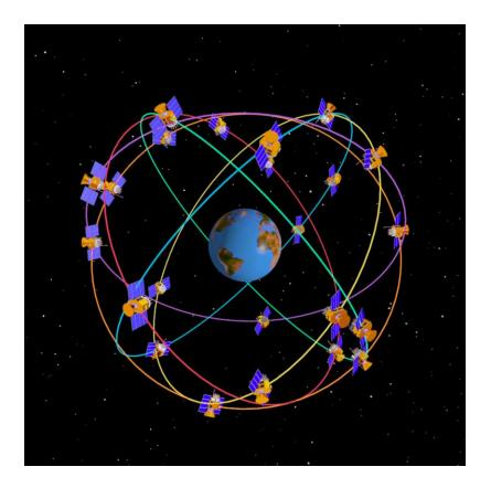
GPS satellites complete an orbit in approximately 12 hours, which means that they pass over any point on the earth about twice a day. The satellites rise (and set) about four minutes earlier each day.
