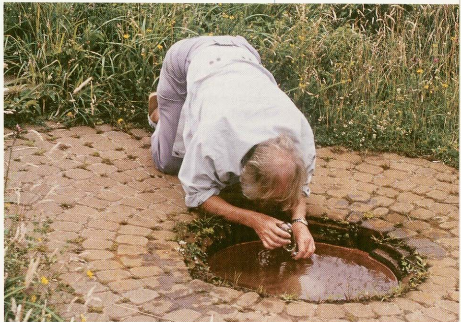
▼ Fig. 13.23. Late Werner Giggenbach, famous gas-geochemist, using the Giggenbach bottle to sample gases rising from a mineral spring in the Eifel (Germany)
