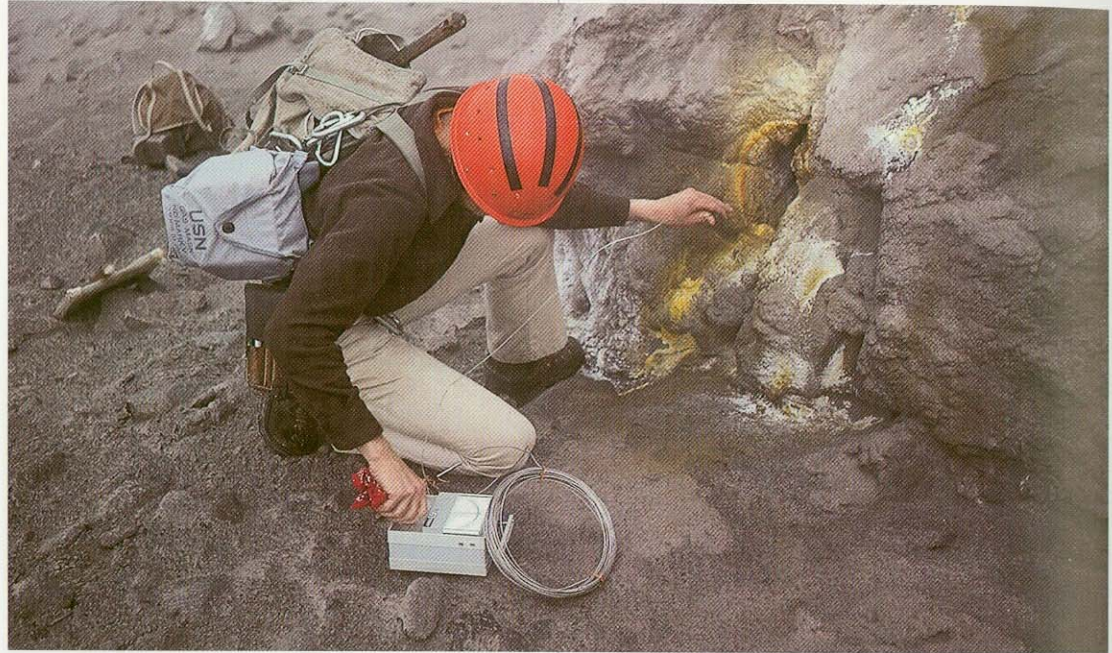
► Fig. 13.24. Measuring temperature in a hot block that traveled with a pyroclastic block flow on the slopes of Augustine volcano in 1976 (Alaska)
