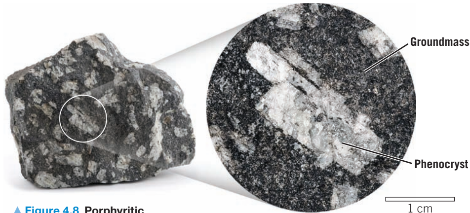
▲ Figure 4.8 Porphyritic texture The large crystals in porphyritic rocks are called phenocrysts , and the matrix of smaller crystals is called groundmass . (Photo by Dennis Tasa)
