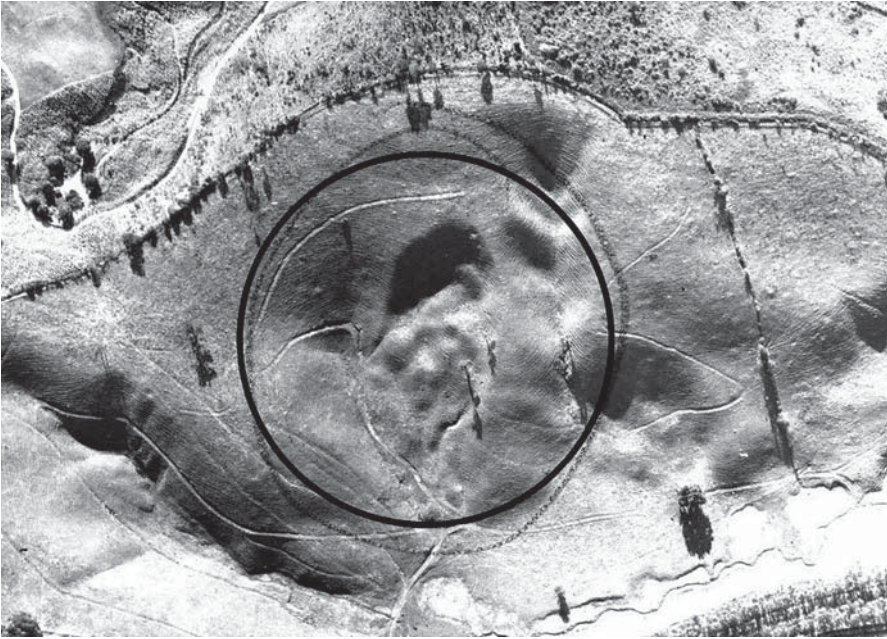
FIGURE 1.27 Old slump slide in residual soils located near slide in Figure 1.26.
