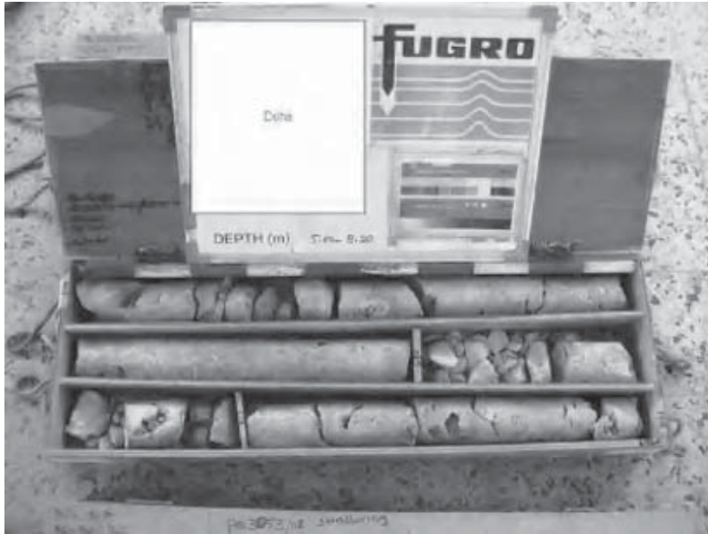
Figure B5-1.3 Example of core through Simsimi Limestone (courtesy of Karim Khalaf, Fugro, Middle East).
