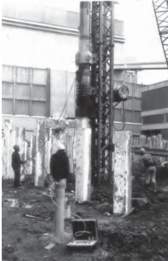
Figure 4.42 Pneumatic piezometer being used to take measurements of rapidly changing water pressures during pile driving. Only small volume changes are necessary to measure pressure changes, so readings could be taken every ten seconds or so. Water pressures measured went off scale at about three times overburden pressure (Hencher & Mallard, 1989), Drax Power Station, Yorkshire, UK.
