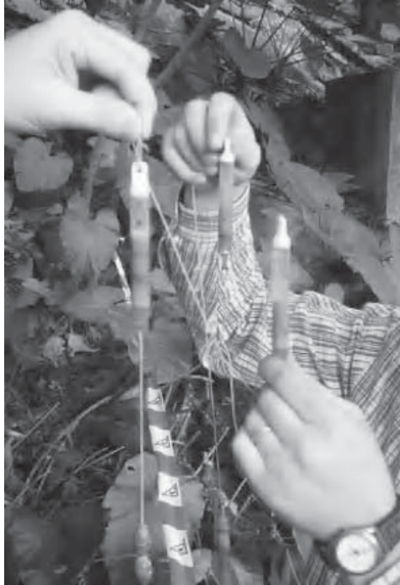
Figure 4.41 Halcrow buckets retrieved at Yee King Road landslide investigation (Hencher et al. , 2008). These are unusual in that they contain sediments (from turbulent flows down the borehole). Normally, they would just contain water (or not), indicating the highest level that the water has risen in the borehole between inspections. Left side bucket is attached by fishing line to lead weights used to lower the buckets down the borehole.
