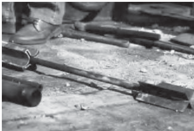
Figure 4.33 Field vane used for measuring strength of clay down borehole or sometimes pushed from the ground surface. Once at test location, the vane is rotated to measure shear strength of the cylinder of soil defined by the vane geometry. To the left is a sleeve used to protect the vane during installation.
