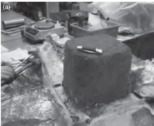
Figure 4.12 (a) Block sample cut into grade IV weathered sedimentary rock and transported to the laboratory. (b) The sample trimmed by hand to fit into a Leeds direct shear box.
