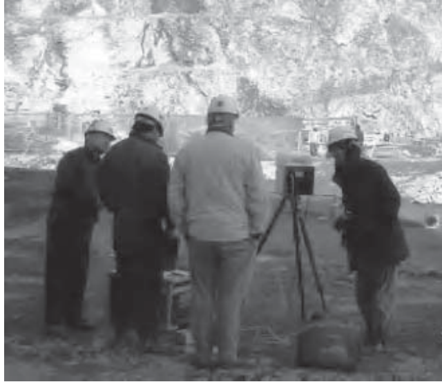
Figure 4.19 Ground-based radar being used to generate a digital image of cut slopes near Seoul, Korea. Point clouds can be used to measure discontinuity geometry remotely.
