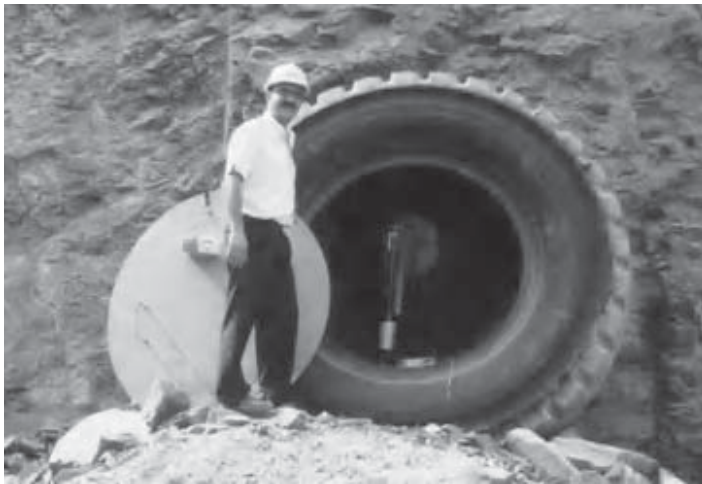
Figure 4.42 Pneumatic piezometer being used to take measurements of rapidly changing water pressures during pile driving. Only small volume changes are necessary to measure pressure changes, so readings could be taken every ten seconds or so. Water pressures measured went off scale at about three times overburden pressure (Hencher & Mallard, 1989), Drax Power Station, Yorkshire, UK.
