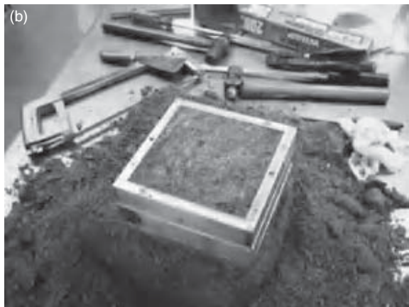
Figure 4.12 (a) Block sample cut into grade IV weathered sedimentary rock and transported to the laboratory. (b) The sample trimmed by hand to fit into a Leeds direct shear box.
