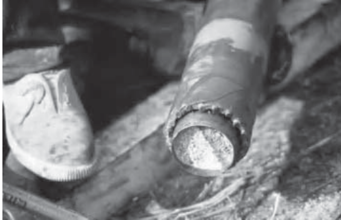
Figure 4.28 Mazier sampler with nicely recovered weathered granite – the right side third is stained with iron oxides. Spring-loaded cutting shoe is seen extending from the rock cutting bit outside. When the material strength becomes too high for the cutting shoe (exceeds spring stiffness), the outer bit takes over the cutting.
