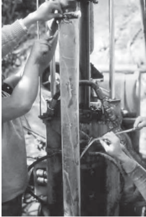
Figure 4.37 Impression packer. Paraffin wax paper has been pushed against the walls of the borehole by a rubber inflatable packer. A series of pale-grey traces can be seen, which represent a set of fairly planar joints dipping at about 70 degrees. Direction is obtained from a compass set in glue at the base of the packer. Other options for orienting devices now include flux gate magnetometers and gyroscopes.
