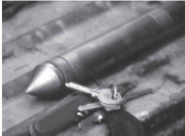
Figure 4.34 Electric static cone penetrometer with piezometric ring. Forces on the cone tip are measured independently from the force on the shaft section above. A combination of all three measurements (including water pressure) gives a good indication of soil type as well as strength characteristics.
