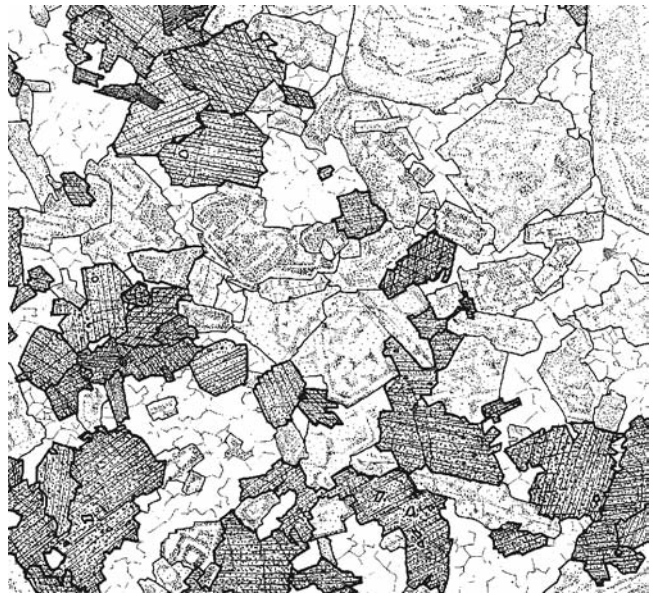
FIGURE 1 Interlocking texture in a granodiorite. From Bard (1986). Copyright © by permission Kluwer Academic Publishers.
