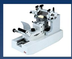
The block holder is mounted on a steel carriage which slides backwards and forwards on guides against a fixed horizontal knife.
