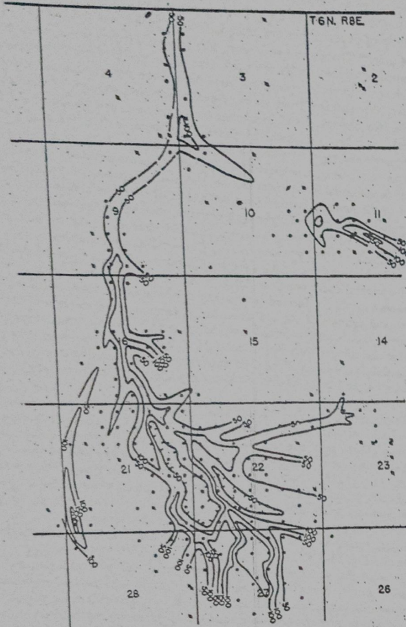
FIGURE 3-5 Isopotential map showing the initial daily rate of oil production in the Hawkins field, Hughes County, Oklahoma. The contour interval is 50 barrels per day. Compare with Figure 13-5, an isopach map of the producing sand of the area. [By the courtesy of Daniel A. Busch.]
