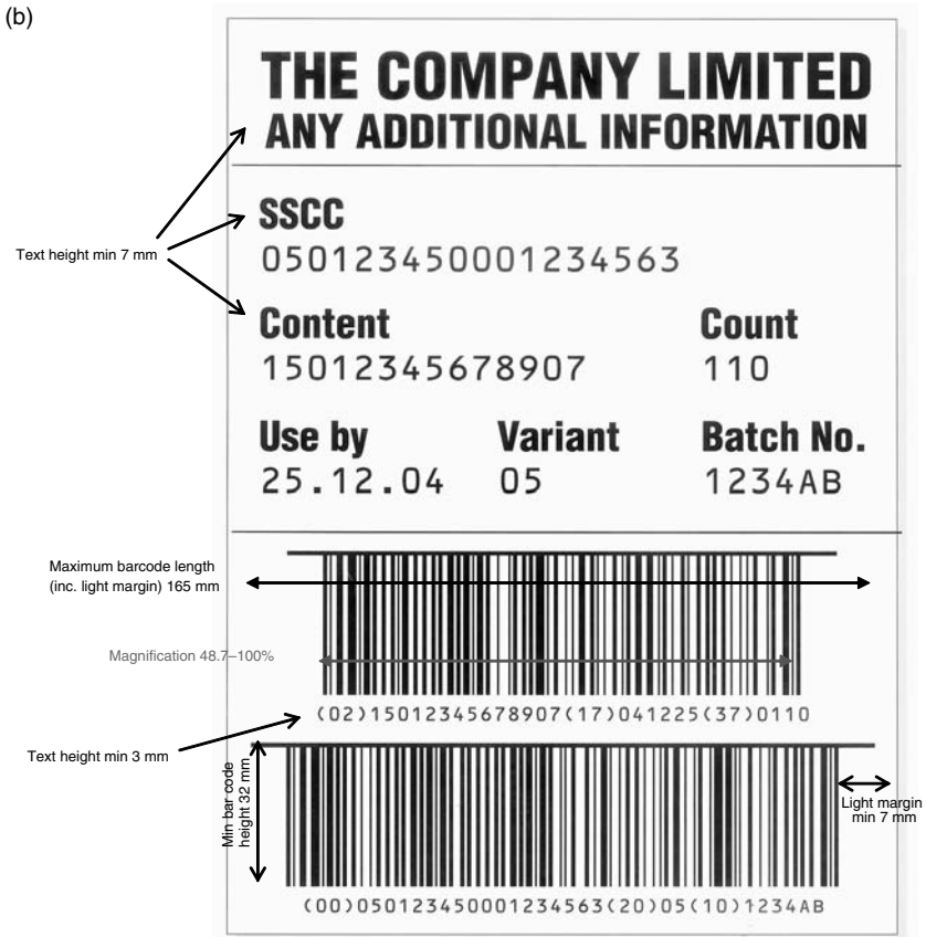
Figure 10.12 Typical barcode label: (a) ITF-14 bar code illustration, (b) EAN-128 bar code illustration.
