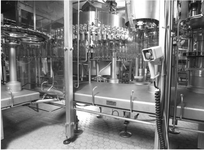
Figure 6.23 Filler showing easily cleanable surfaces (courtesy Kronos UK Ltd).
