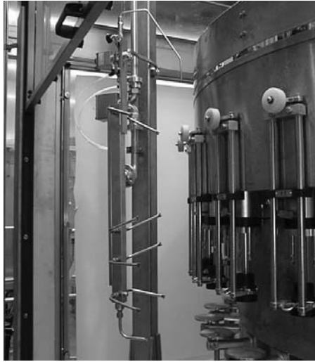
Figure 6.12 Bottles on the filler carousel sealed against centring bells (courtesy Kronos UK Ltd).
