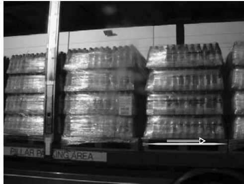
Figure 8.21 Reject load (courtesy British Soft Drinks Assoc.).
