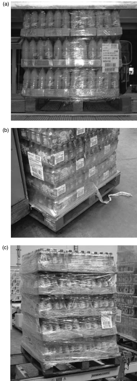
Figure 8.20 Poor palletisation. (a) Load offset on pallet, (b) stretch wrap tail, (c) loose stretch wrap, (d) load shifted on braking, (e) multiple pallet labels, (f) effect of severe braking, (g) bad stacking of mixed load, and (h) typical mixed cage (courtesy Linpac).
