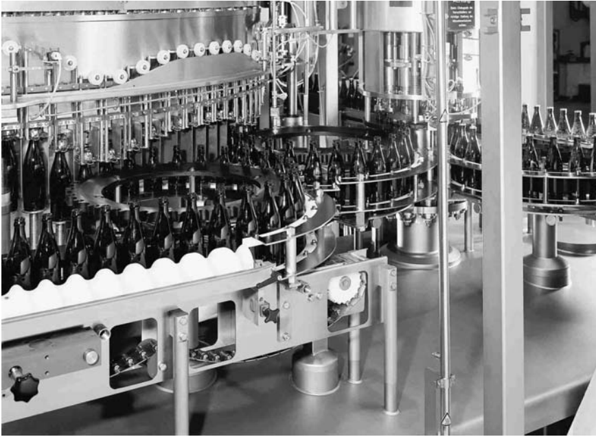
Figure 6.9 Bottle transfer in filler (courtesy Krones UK Ltd).
