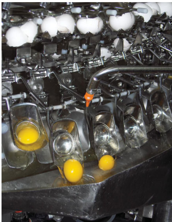
Figure 19.4 Eggs are first cracked and egg contents fall into a yolk-albumen separator where the top cup retains only yolk while whites slide to the bottom cup. Courtesy of Dr Vincent Guyonnet of Burnbrae Farm Ltd., Canada.
