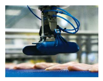
Marel Multihead Weighers handle all in-feed, sorting, mixing and weighing requirements. They automatically portion and pack all types of fresh or frozen poultry products.
