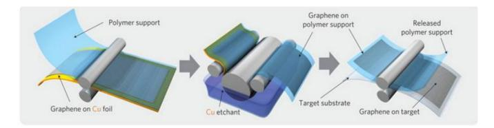
Roll-to-roll manufacturing could allow graphene to be made at large scales. Korea University
