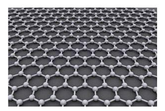
Carbon is an incredibly versatile element. Depending on how atoms are arranged, it can produce hard <u>diamonds or soft graphite</u>. Graphene's flat honeycomb pattern grants it many unusual characteristics, including the status of <u>strongest material in the world</u>.
