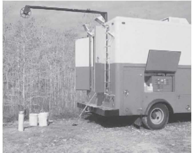
Figure 3. A typical logging truck used in shallow subsurface investigations; the truck is equipped with 1500 m of wireline, winch, generator, digitally controlled operating system, and probes capable of making most of the geophysical measurements listed in Table 1.
