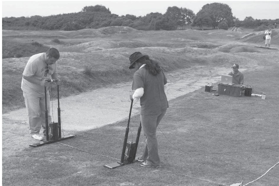
Figure 9.13 In-line 100 MHz GPR data acquisition with a 1.0-m TX–RX separation distance.
